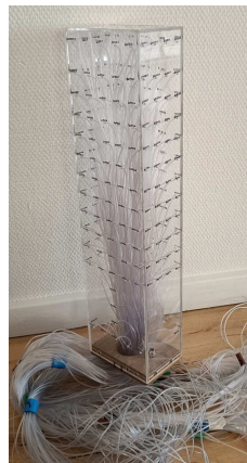
Figure 2. Photo of the applied scale pressure model of the CAARC building.
